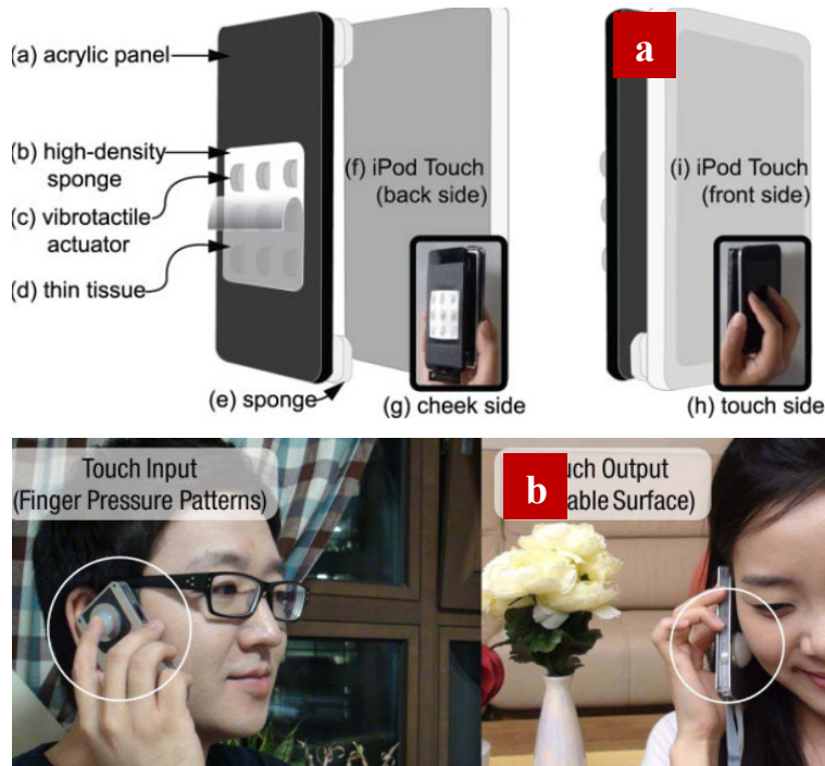
Figure 2.31. a. Vibrotactile display on a mobile phone by Park et al. (2012), and b. POKE by Park et al. (2013)
